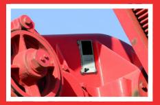
Attach the ViaSat-10 to a metallic surface on the asset
