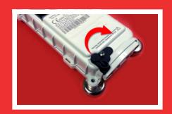
Remove the magnetic grommet to power-on the ViaSat-10
